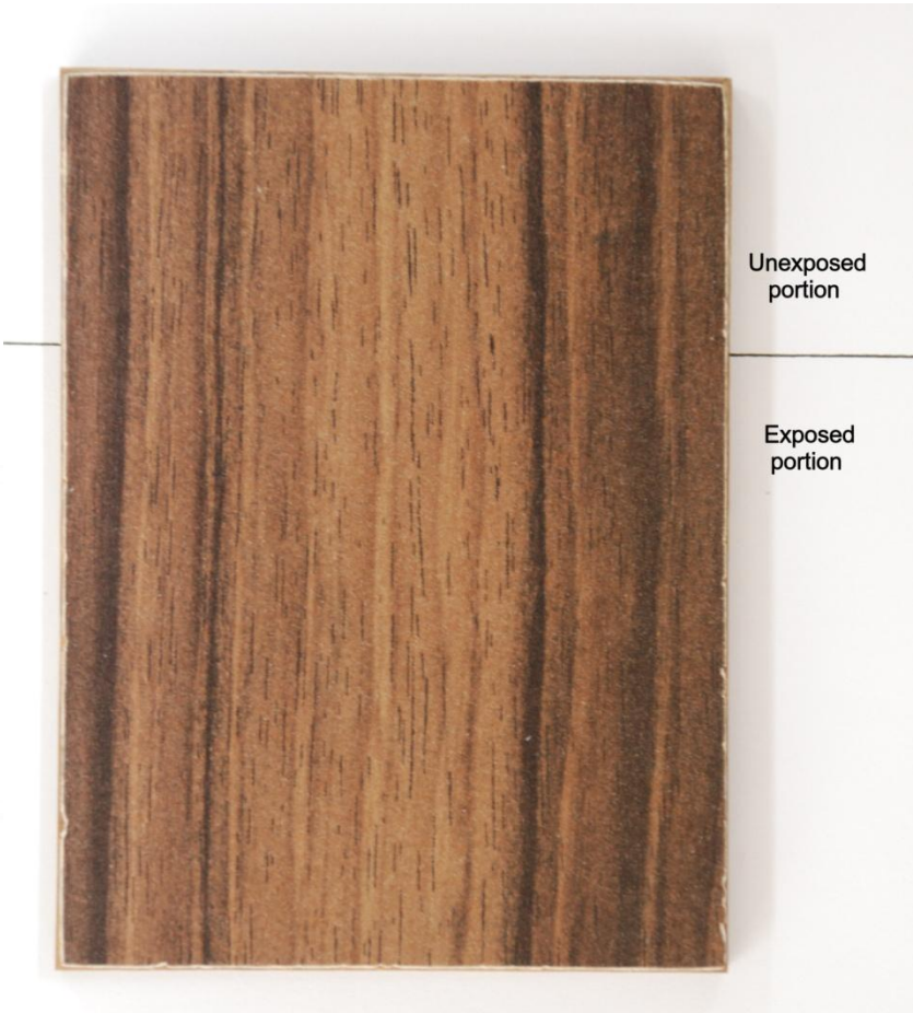
“Greenlam CLADS™ Exterior Grade Compact Laminates” After Lightfastness (Xenon arc) Test
